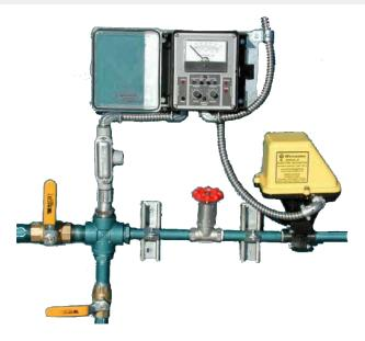
Automated surface blowdown systems utilize a controller, conductivity sensing probe, and motorized ball valve to test boiler water properties and then blowdown if needed. This is typically set up to run every hour, blowing down only if conductivity is high.
