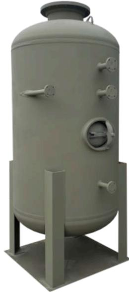
The boiler room has many hot, high pressure water lines that often need a safe place to be discharged to. The blowdown process is relatively violent and yields flash steam. ASME Pressure vessels are sized and used to safely contain and cool this process.
